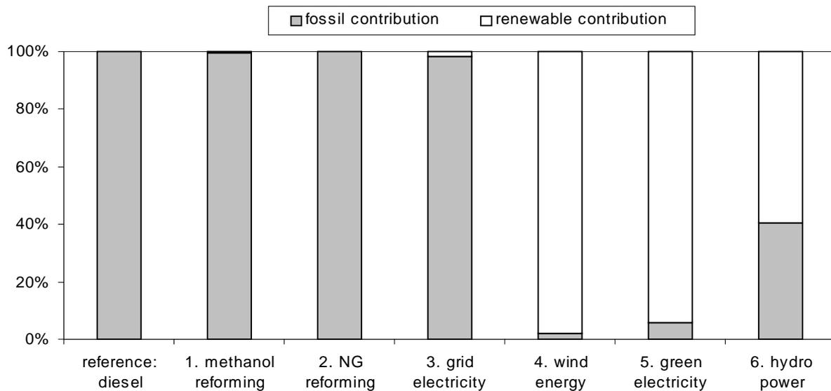
**Figure 2:** Cumulated energy in kWh primary energy per 100 kilometres; same data as in Figure 1 but differentiated with regard to the sources of primary energy and displayed in relative terms. A third category of minor importance is omitted here for clarity (cf. main text).
