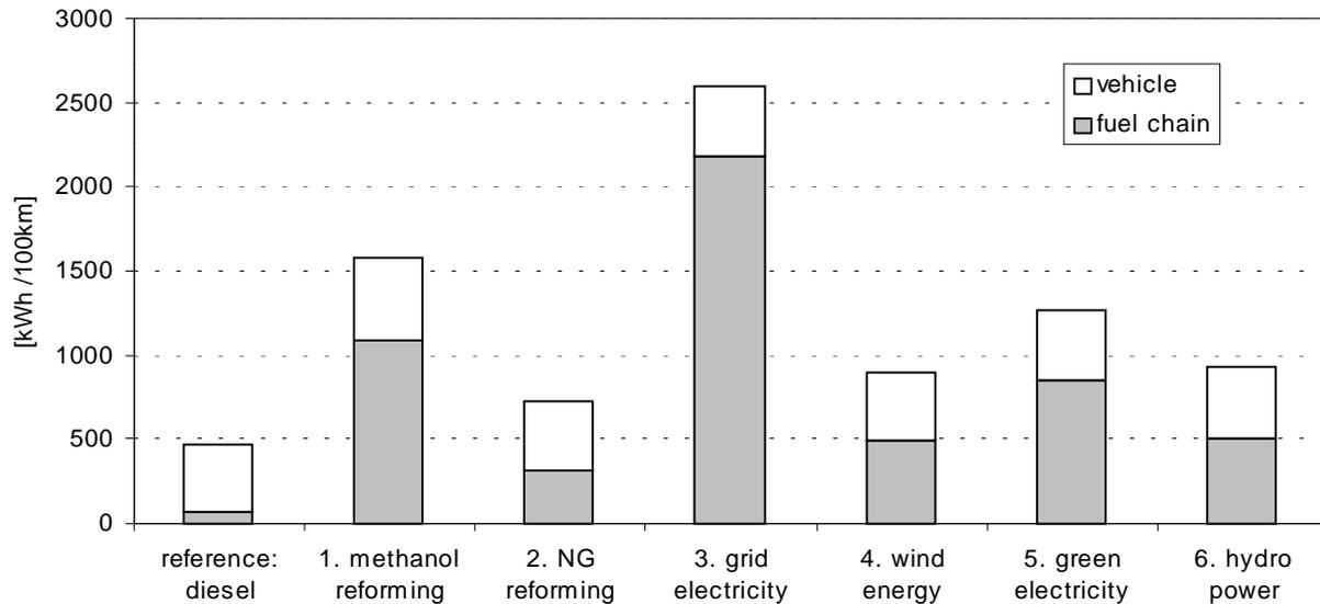
**Figure 1:** Cumulated energy “from well to wheel” in kWh primary energy per 100 kilometres. The dark sections of the bars depict contributions from the fuel chain. The light parts denote fuel consumption on board of the vehicle. “NG” stands for natural gas.
