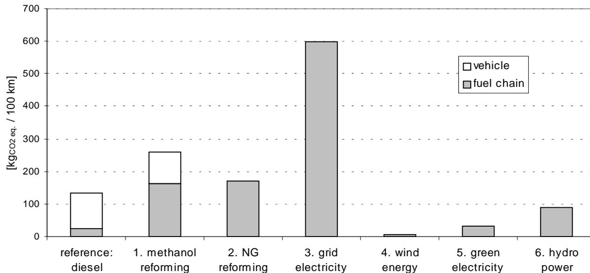
**Figure 3:** Carbon dioxide equivalent emissions for the scenarios as in Figure 1. Again, the dark parts of the bars depict contributions from the fuel processing chain, the light parts stand for emissions from the vehicle itself. As fuel cells only emit water vapour, the vehicle contribution is zero in all hydrogen scenarios except for the case of on-board methanol reforming.
